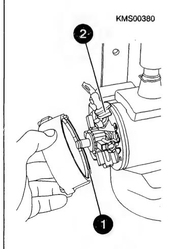
Assembling commutator end shield
